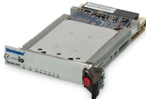
StoreEngine Air Cooled SE306-VPX is shown with one optional StorePak XMC (SSD storage) module
