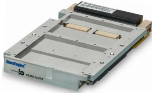
StoreEngine 3U Conduction Cooled VPX SE300-CCVPX-ND accommodates standard I/O XMCs
