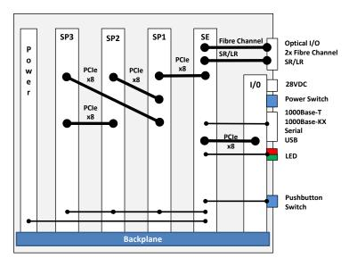
The SB1C4-F08 RAID/recorder architecture combines StoreEngine's high-performance recording and storage management software with up to three hot-swappable StorePak modules to provide up to 18TB of solid state storage in a compact, lightweight, rugged conduction cooled chassis
