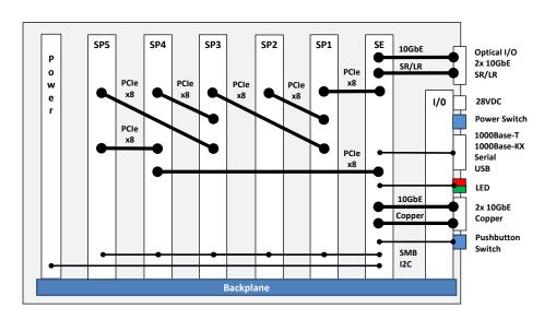
The SB1C6-E10 recorder architecture combines StoreEngine's high-performance recording and storage management software with up to five hot-swappable StorePak modules to provide up to 30TB of solid state storage in a compact, lightweight, rugged conduction cooled chassis
