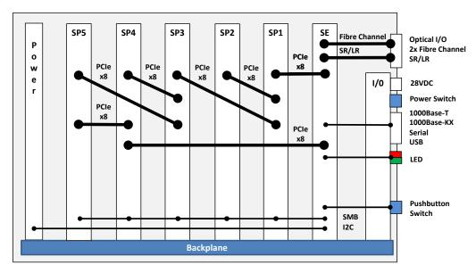
The SB1C6-F08 RAID/recorder architecture combines StoreEngine's high-performance recording and storage management software with up to five hot-swappable StorePak modules to provide up to 30TB of solid state storage in a compact, lightweight, rugged conduction cooled chassis
