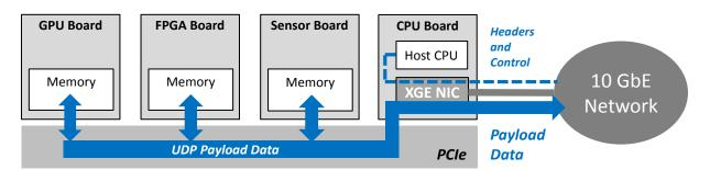
The UDP Direct stream mode of operation can be used concurrently with general purpose 10GbE netwok traffic using the normal network stack. The XGE NIC hardware, firmware, and driver software support simultaneous usage for UDP direct stream transfers and standard networking.
