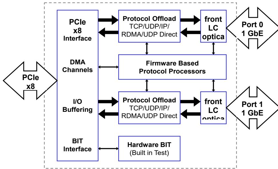
**Block Diagram:** Functional block diagram for the XGE4044 XMC by Critical I/O. This XMC provides two independent 1 Gb Ethernet ports, each with integrated protocol offload hardware. Dedicated hardware offload provides full duplex operation at wire-speed, up to 250 MB/s (per port).
