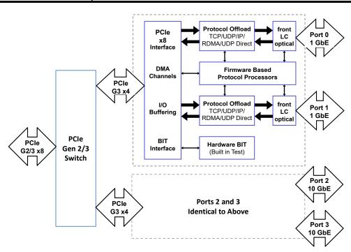
**Block Diagram:** Functional block diagram for the XGE4140 XMC by Critical I/O. This XMC provides four independent 10 Gb Ethernet ports, with integrated protocol offload hardware. Dedicated hardware offload provides full duplex operation at full wire-speed, up to 2500 MB/s (per port).
