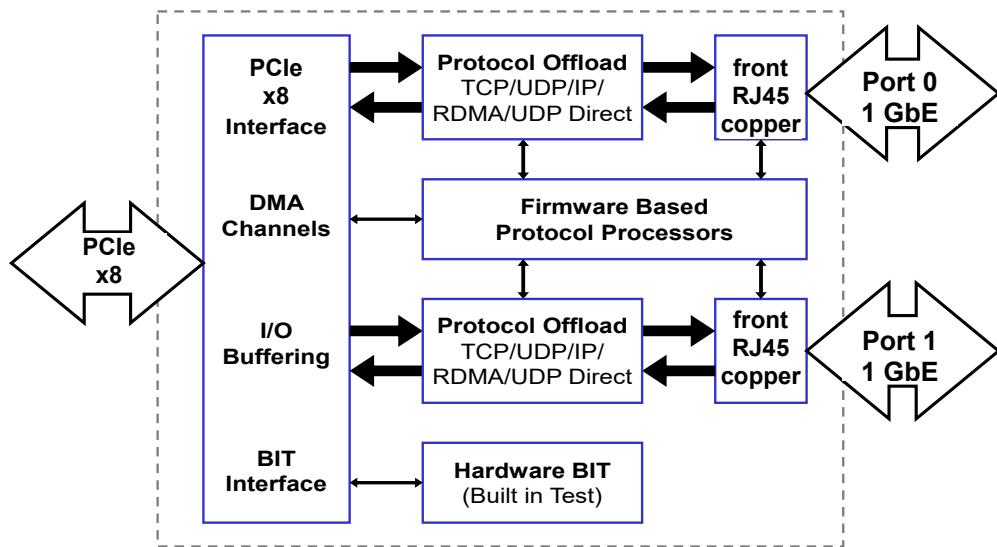
**Block Diagram:** Functional block diagram for the XGE4043 XMC by Critical I/O. This XMC provides dual independent 1 Gb Ethernet ports, each with integrated protocol offload hardware. Dedicated hardware offload provides full duplex operation at wire-speed, up to 250 MB/s (per port).
